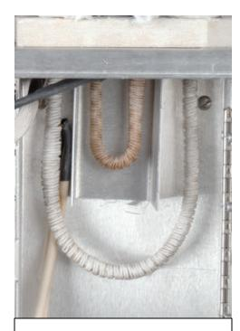
Stratum PTC Newly Designed Ushaped Analytical and Condensate Traps
