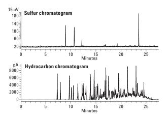
Figure 2. JP-4 FID/SCD chromatogram with internal standard (split 1:10).
