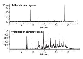
Figure 1. Simultaneous FID/SCD chromatogram of JP-4 (split 1:10).
