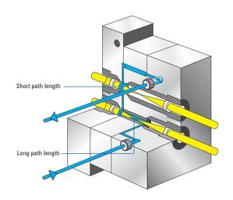
Achieve up to 80 AU when moving from analytical to preparative operation, without changing the dual path-length flow cell. Above shows dynamic range from 2 to 21 AU of 5-hydroxytryptophan sample.
