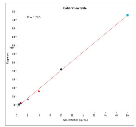
Figure 6 Calibration of 1290 Infinity 2D-LC Solution for resveratrol quantification, 1–50  $\mu$ g/mL found in merlot: 4.5  $\mu$ g/mL, 4.5 mg/L.
