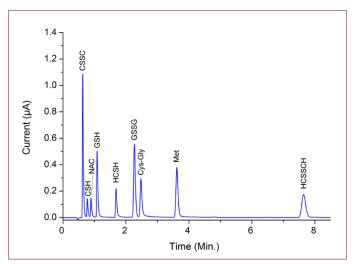
Figure 3: Chromatogram of a 1  $\mu$ L injection of 10  $\mu$ mol/L standard mix diluted in mobile phase: Cystine (CSSC), Cysteine (CSH), N-acetyl Cysteine (NAC), Glutathione (GSH), Homocysteine (HCSH), L-Cysteine-L-Glycine (Cys-Gly), oxidized Glutathione (GSSG), Methionine (Met) and Homocistine (HCSSCH).
