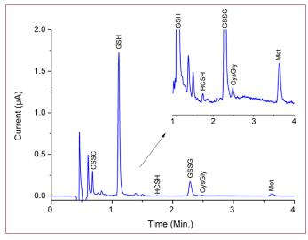
Figure 8: Chromatogram obtained from a 1 μL injection of a whole blood sample. Top-right inset: zoom-in on response of HCSH, CysGly and Met.
