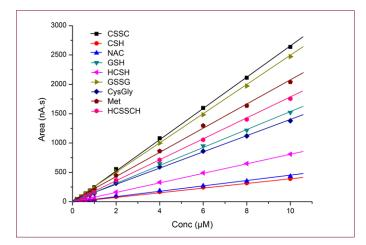
Figure 4: Calibration curves for all 9 aminothiols and disulfides dissolved in mobile phase (concentration range 0.2 – 10  $\mu$ mol/L).
