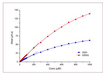
**Figure 5:** Calibration curves for reduced (GSH) and oxidized Glutathione (GSSG) in the concentration range  $10 - 1000 \, \mu mol/L$ .
