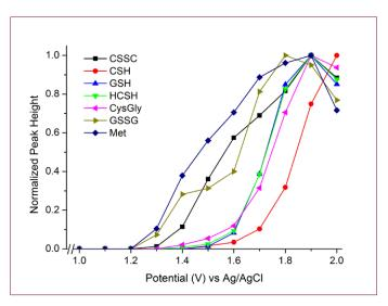
Figure 2: Voltammograms of 10  $\mu$ mol/L standards using potentials between 1 and 2 V.
