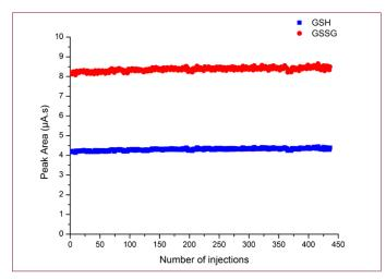
**Figure 6:** Long-term repeatability of DC amperometric detection of reduced (GSH) and oxidized (GSSG) Glutathione on a diamond working electrode. Sample concentration 50  $\mu$ mol/L, injection volume 1  $\mu$ L.
