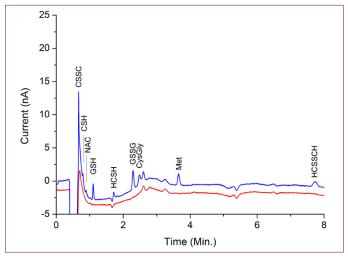
**Figure 7:** Overlay of a blank (red trace, 0.5 mol/L PCA) and a chromatogram of a 1  $\mu$ L injection of 50 nmol/L standard mix diluted in 0.5 mol/L PCA (blue trace): Cystine (CSSC), Cysteine (CSH), N-acetyl Cysteine (NAC), Glutathione (GSH), Homocysteine (HCSH), L-Cysteine-L-Glycine (Cys-Gly), oxidized Glutathione (GSSG), Methionine (Met) and Homocistine (HCSSCH).
