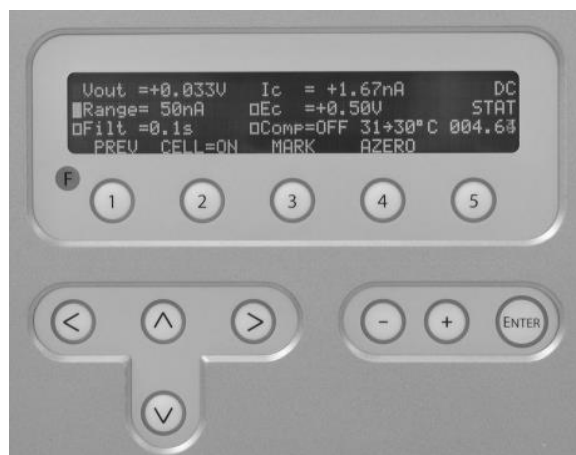
Fig. 4. DECADE II keyboard. The cursor is on 'Range' which allows changes using the value buttons '+' and '-'. The 'Enter' button is only used to confirm changes in potential ( E_c ).
